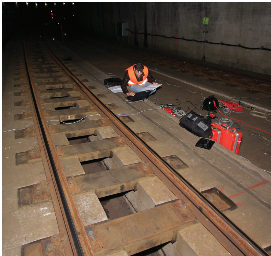
Measuring equipment in the measurement section with mass-spring system (MSS)
